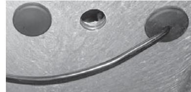
Push the connector through the mounting bracket in the inlet chamber. Please keep in mind that the level switch must be rotated 180 degrees in regards to the gravity position! Then put the nut over the connector and screw it on the level switch.
