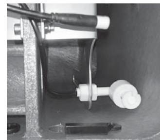
Push the connector through the opening and push it through the rubber plug. The small hole of the plug can be widened with a sharp knife to make this a little easier. Put the plug in the middle opening.
