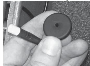
Remove the level switch from the drum chamber by taking the nut and connector through the mounting bracket.
