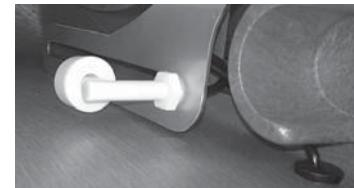
Take out the rubber plug from the housing and pull out the level switch connector. Push the connector through the rubber plug so it is free.
