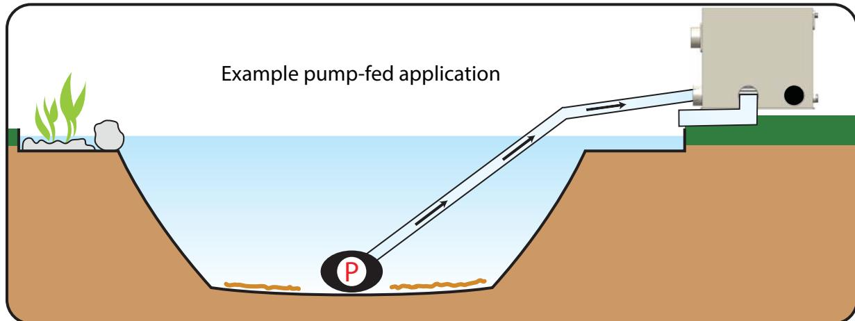
For pump fed application you must change the position of the level switch from the drum chamber mounting bracket to the inlet chamber mounting bracket (see next page for detailed instructions). For pump fed application the level switch must be rotated 180 degrees (see illustration). In a pump fed application you can adjust the socket height of the overflow pipe. This overflow pipe will allow (unfiltered) water to flow into the drum chamber and back to the pond in case of a malfunctioning.
