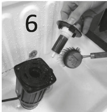
Clean rotor with water and brush
