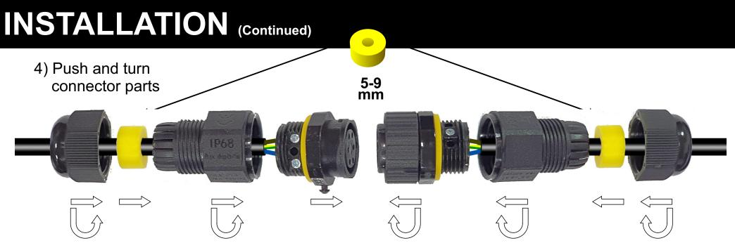
5) To lock, align the arrow style pins and the small tab on the central ring and push together
