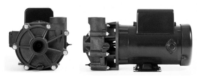
PerformancePro Pumps are end suction centrifugal units that close couple to 56J motors. They are molded of Noryl or Polypropylene for excellent corrosion resistance. Both suction and discharge ports are 1 1/2" female NPT.
