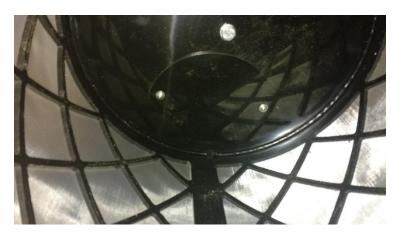
If you need to bypass the drum, for instance if you are treating for flukes, there is a bypass plate that can be removed from inside the drum itself and is secured by 2 self tapping screws. This is accessed by removal of the waste tray.
